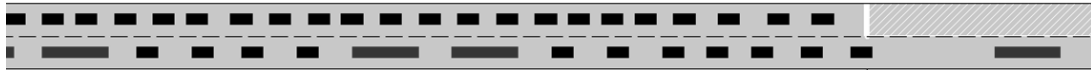
Figure C.1 – Screenshot of SIMBA near the lane closure showing plan view of traffic (small black bars = cars; longer gray bars = trucks; white line = closure).
