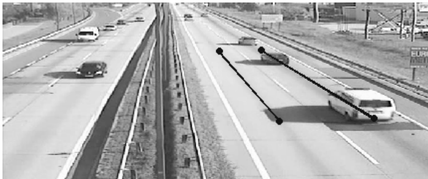
Figure E.15 – Detection lines (after Mirth (2008)).
