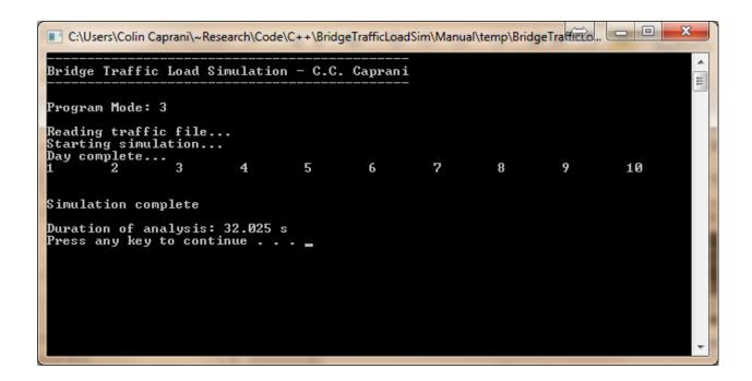
Note the slower execution time than for Program Mode 1 which has 20 days of traffic. This is caused by the additional overhead required to manipulate the 25 MB traffic file that has been read into memory.
